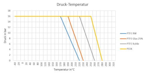
By ignoring these limit values, improper use of the compact- valve is the consequence and could lead to failure of the valve function.
