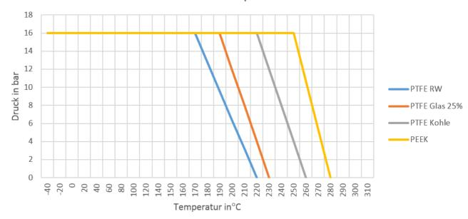
By ignoring these limit values, improper use of the compact-valve is the consequence and could lead to failure of the valve function.
